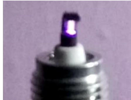
Gambar 10. Bunga api busi U20EPR9 dimana R1=3.3k , R2=3.3k C1=10\mu F
