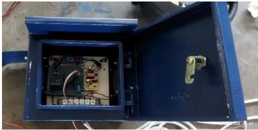
Gambar 4. Rangkaian elektronik alat Early Warning System bencana banjir
